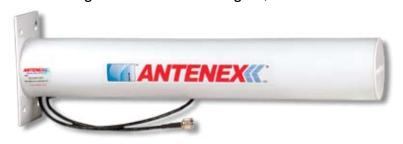
air filled radome yields a higher efficiency and greater performance than the stamped or printed circuit versions. This entire antenna package is 1.6 lbs. and comes with an 18" pigtail of low loss coax cable terminated with an N female connector. The YE series has a VSWR of <2.1:1 from 2.4 GHz to 2.48 GHz and can be mounted outdoors in even the most harsh weather conditions.
