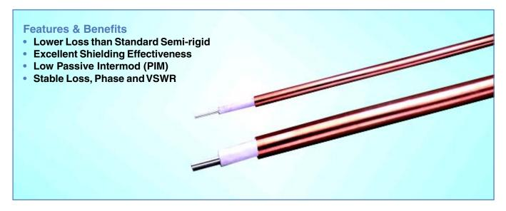
**Coppersol-CLL** employs a thin tubular copper outer conductor and low-density PTFE dielectric which provide the lowest loss and highest shielding giving it significant performance advantages over semirigid coax of similar size.
